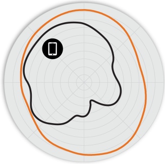
Figure 2. H550 2.4GHz Azimuth Antenna Patterns
