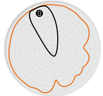
Figure 5. H550 5GHz Elevation Antenna Patterns
